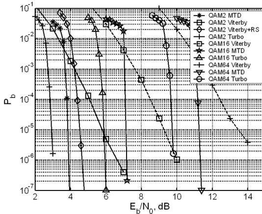
Fig. 1. Performance of MTD over AWGN channel with QAM
